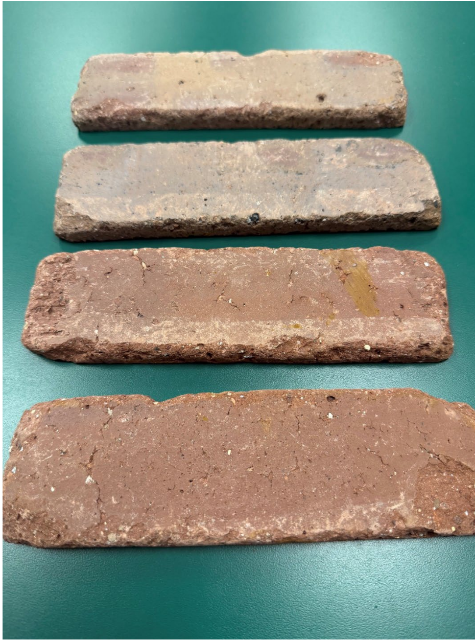
Bricks Proposed for Reconstructed Chimney
