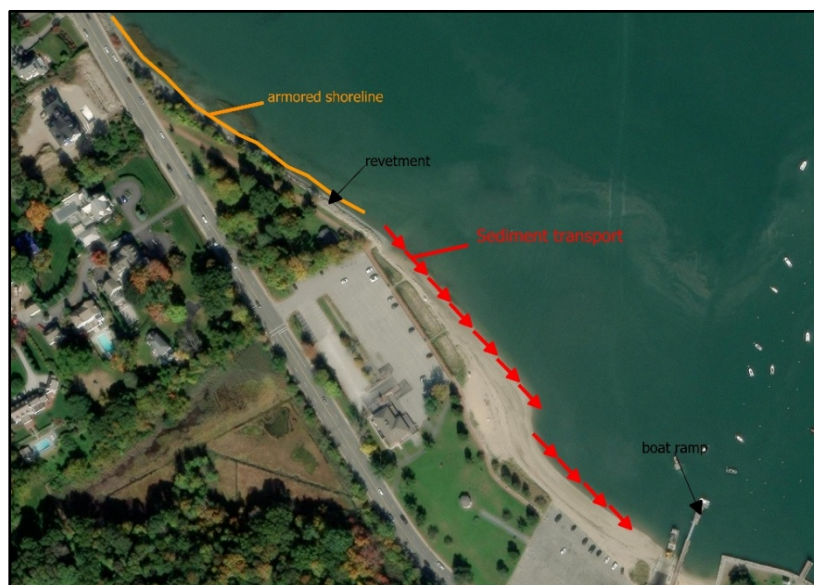
Figure 15: Predominant direction of wave-induced littoral drift (northwest-to-southeast) is illustrated by the red arrows, providing limited natural nourishment for Bathing Beach. Additionally, armored shorelines (orange) directly updrift from the beach restrict sediment inputs. The result is a closed littoral system with its terminus at the Town boat ramp.
